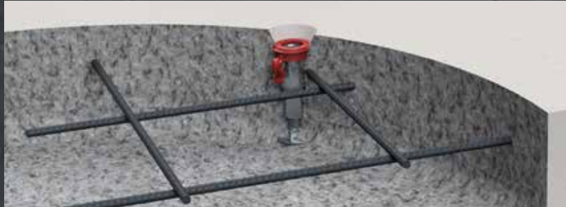
Diagonal tension WITHOUT additional reinforcement
