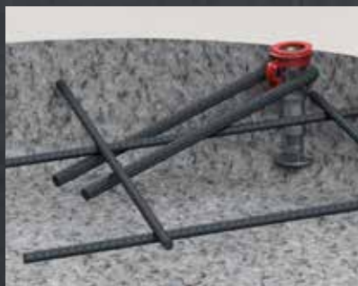
Diagonal tension WITH additional reinforcement
